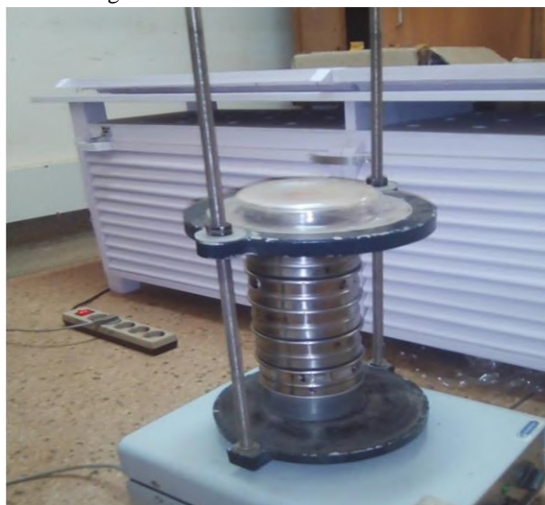
Fig.3.4: Mechanical shaker and sieves
