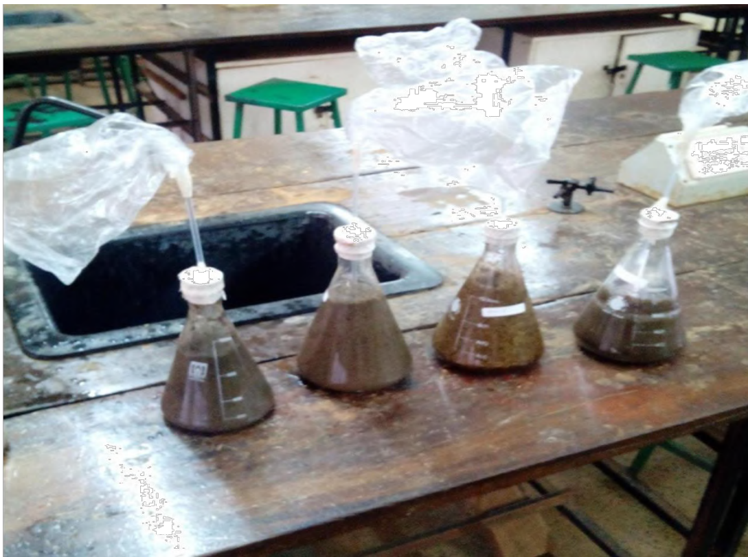
Fig.2.5: Set up for biogas production
