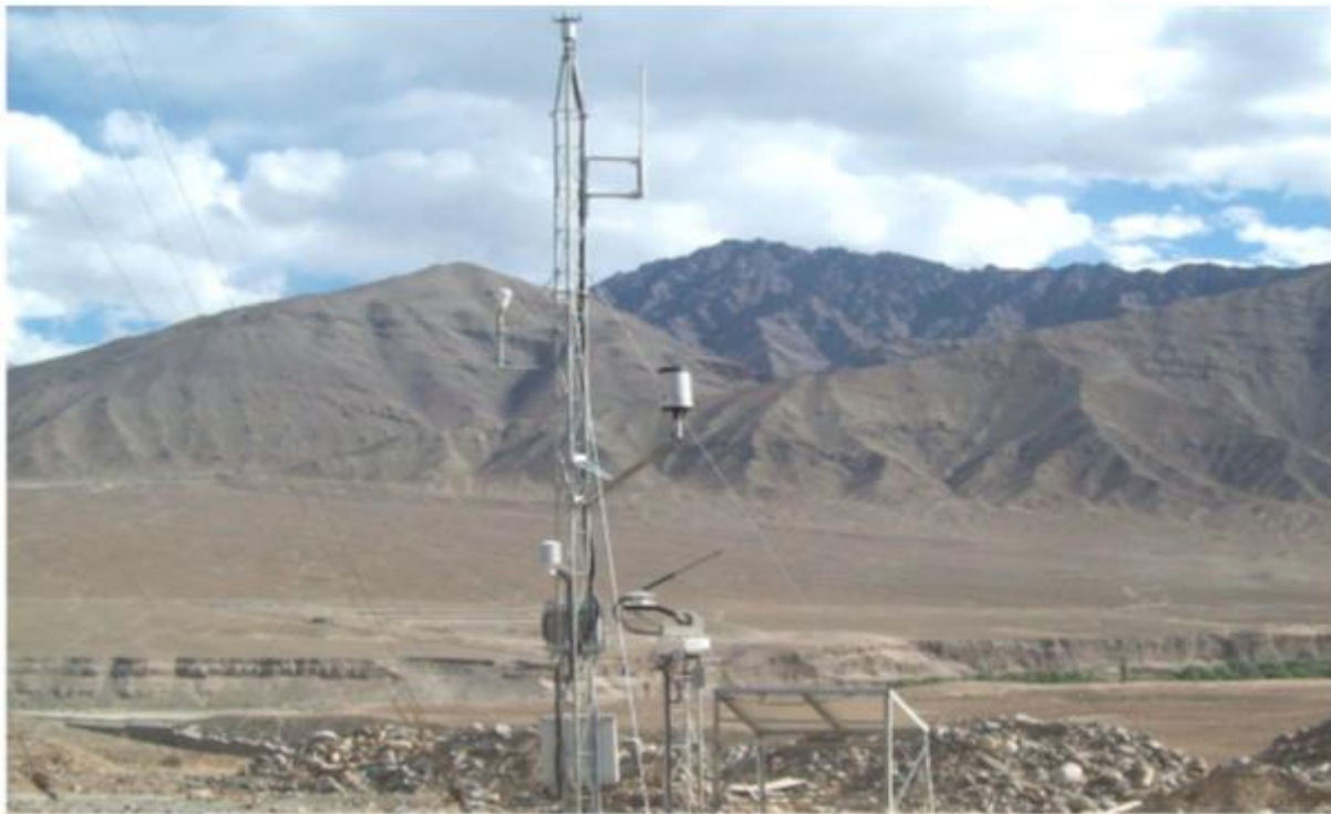
Fig.2: SRRA station by Centre of Wind Energy Technology (MNRE) at Leh for assessment of solar radiation data.
